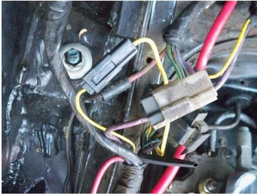
Connect the jumper into that housing
