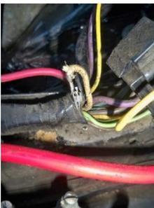
Remove the braided resistance wire at the main terminal. Fold it over 180 degrees. Shrink tube over it, or tape it up.
