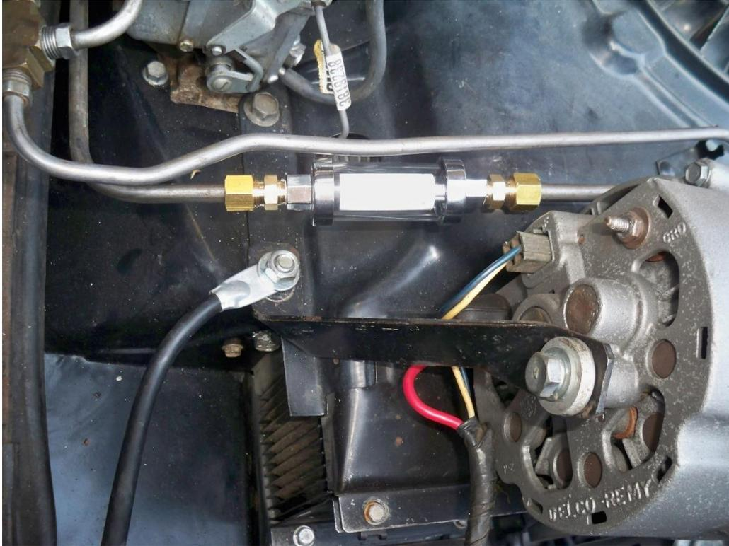
8) Start the motor and look for any leaks - either fuel out or air in. And watch the fuel flow. Look for any crud to be captured by the element.
