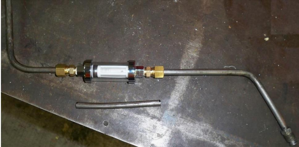
4) Install the filter onto the installed fitting/tube. Lay the other portion in place, adjust it to the marked points. And mark the tube.
