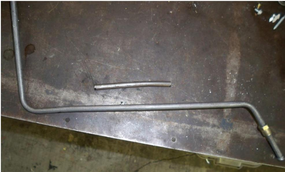
2)Slide the tube nut and the ferrule on - Don't forget this part!
