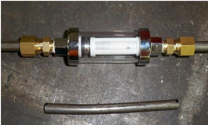
7) Do final assembly and install on the car. I did the final tightening after the tube was in place. Use pairs of wrenches to support each fitting as you tighten. Avoid twisting the whole line
