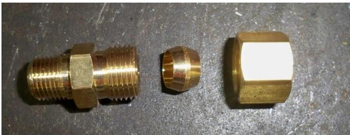
3)Install the adapter fittings onto the filter ends – Pipe threads, use sealer if you wish.
